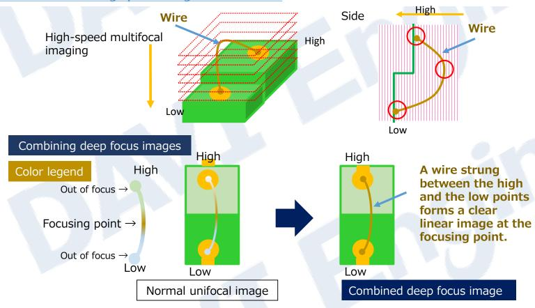
Can detect abnormal wire curves up to \*7.6µm
