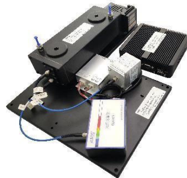
Low density gas inspection module (DOAS)
