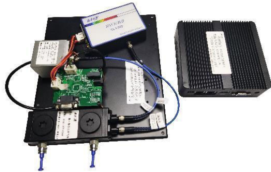
Portable UV gas inspection module (DOAS)
