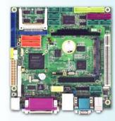
The VDX-6190 /VSX-6190S are the turnkey solution that integrate the Vortex86DX/SX, GPU and DDR2 Memory. Users can easily verify the performance of Vortex86DX/SX processor and it's build-in rich I/O functions like LAN, USB, RS232,GPIO, PS/2, Printer, IDE, WDT, ISA and PCI interface.
