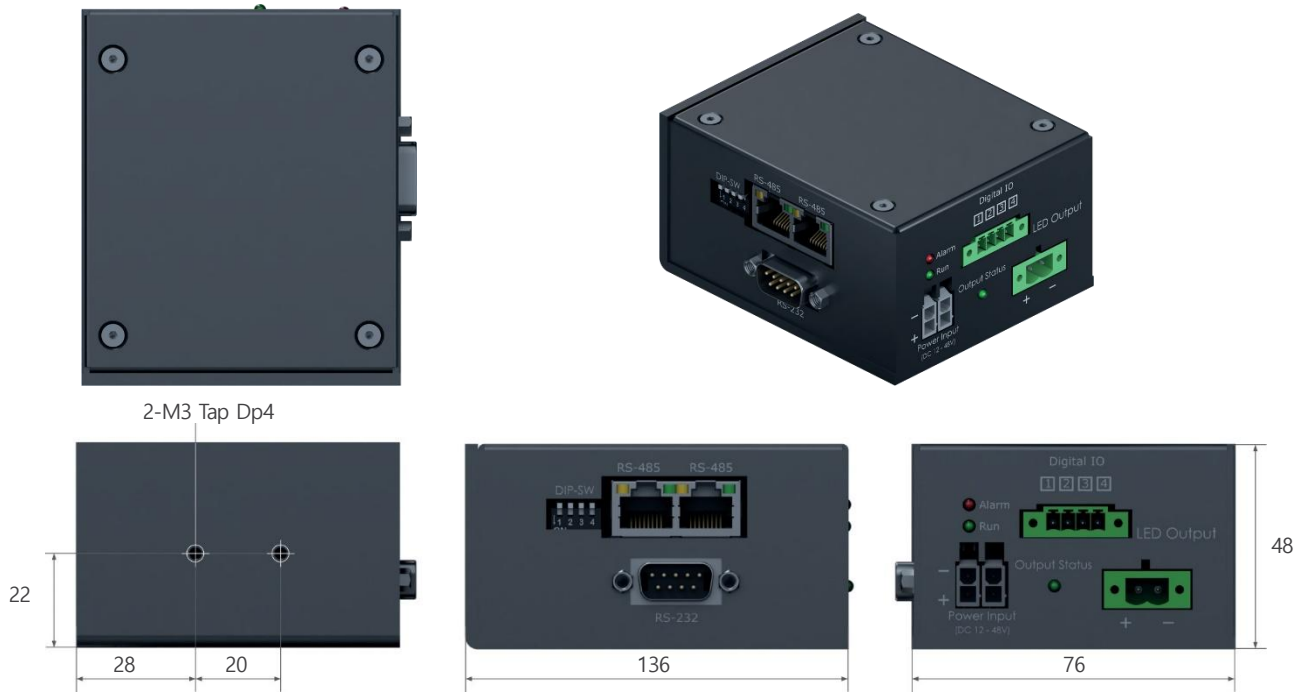
Figure 22 Mechanical Dimension (in mm) for 1 channel strobe controller
