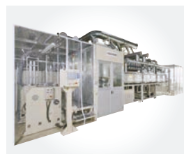
▲ coating drying equipment
