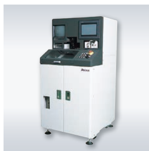
scribing/breaking equipment (LD/LED)
