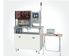
Electrolyte leak inspection equipment
