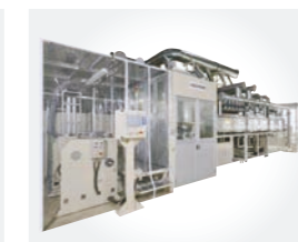
▲ electrode coating & drying furnace
